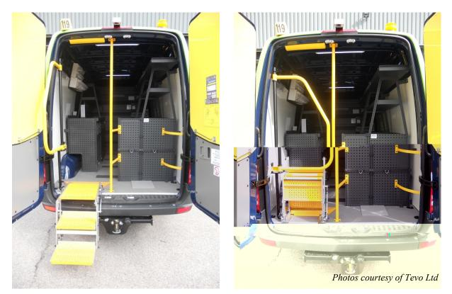
The DM400R step fits at the rear door of a RWD van with sufficient overhang to span the bumper when deployed. It can be mounted either side of the entrance to clear a tow bar hitch.
